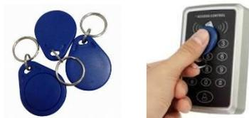
The Tag system uses RFID in Access Control, using radio-frequency electromagnetic fields to identify people of objects without making physical contact. The typical RFID-based controlled access solution consists of tags that contain unique identification data capable of granting or denying access to individuals.
